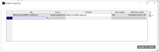
All tags will have system-generated **User Created** and **Date/Time Created** fields added. The Date/Time is based on when the tag was created.
