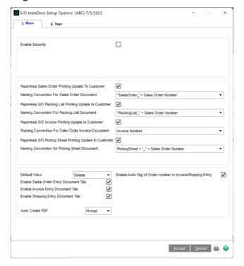
**Enable Security:** Selecting this checkbox turns on the Module Security Options in Role Maintenance. Please refer to the **InstaDocs Security** section in this User Manual.
